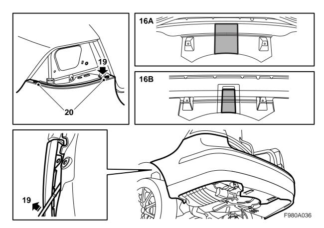
16 Use a universal knife with a hooked blade to cut a hole for the towbar in the bumper shell (a jig saw can also be used).
